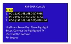
There is a status field for each Transmitter: FREE, BUSY and OFF-LINE. "FREE" means the Transmitter is not used by any user and is available for the keyboard/mouse remote control. "BUSY" means the Transmitter is currently keyboard/mouse controlled by
